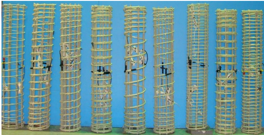
Figure 1: Overview of the of the assembled GFRP cages.
