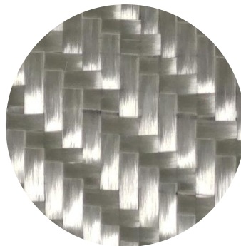
Figure 1. Top view of the glass twill weave reinforcement L1402197.
