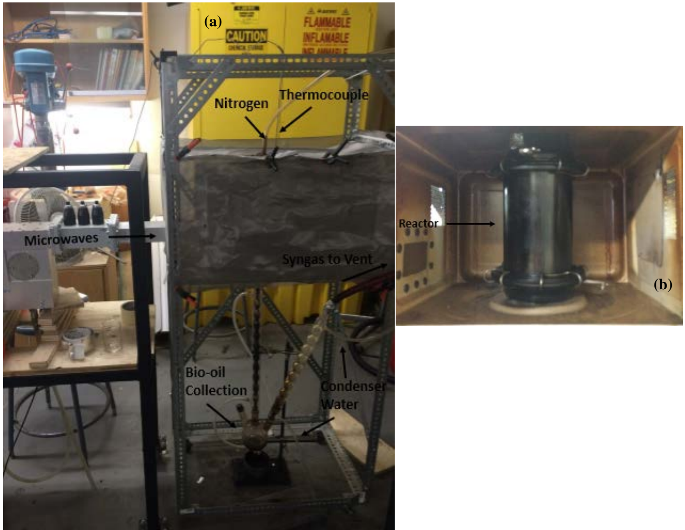
Figure 1: (a) microwave pyrolysis system and (b) reactor used in the experiment.
