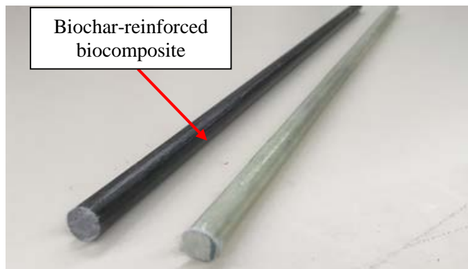
Figure 5: Pultruded biocomposite and conventional GFRP composite rebars.
