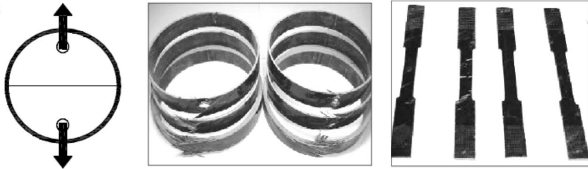
Figure 3. Specimens of FRP tubes for the split-disk test and coupon tensile test [6]
