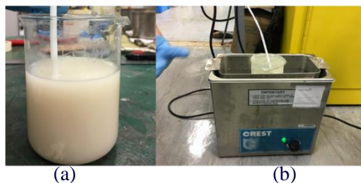
Figure 3. (a) Nanoparticle added to hardener, (b) Stirring the solution
