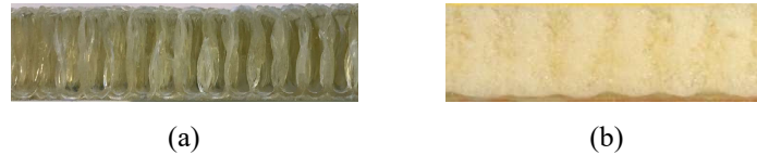
Figure 1. The 3D fiberglass fabric (3DFGF) with its cores (a) without foam, (b) with foam.
