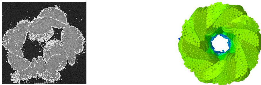
Figure 9: Comparison of the braid cross-sections. a) CT scan cross-section image. b) Braid model cross-section.
