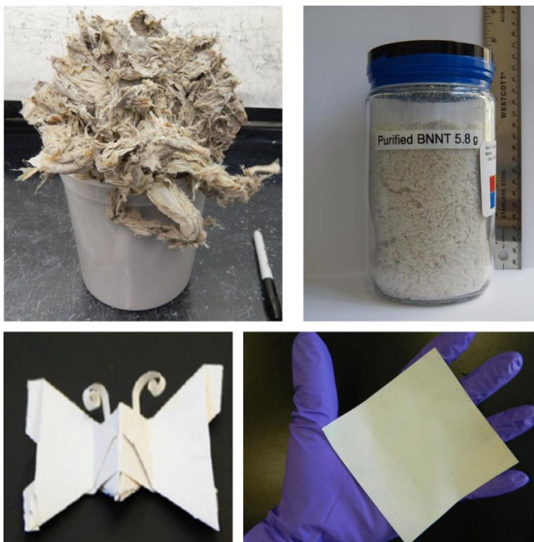
Figure 2. Clockwise from top-left: \sim 20 g of as-synthesized BNNTs [8], purified/homogenized BNNT powder (fluff-like), BNNT buckypaper sheet, and a folded origami butterfly [12]. Reproduced from Jakubinek et al., TechConnect Briefs 2017 with permission (images originally from [8] and [12] are reproduced with permission of The American Chemical Society and The Royal Society of Chemistry, respectively).
