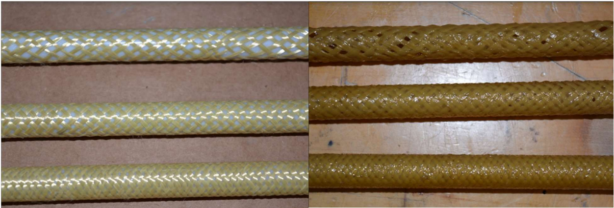
Figure 1: Non-impregnated tubular braided composite yarn preforms (left) and fully-fabricated braided composite tubes impregnated with a resin matrix (right)
