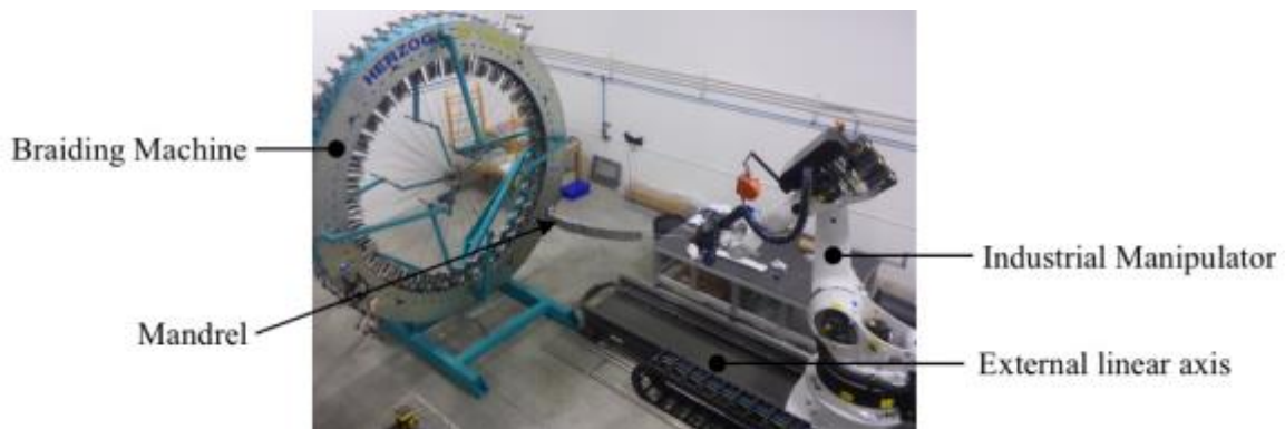
Figure 4. Automated braiding system composed of a Herzog radial braiding machine and a KUKA industrial manipulator.
