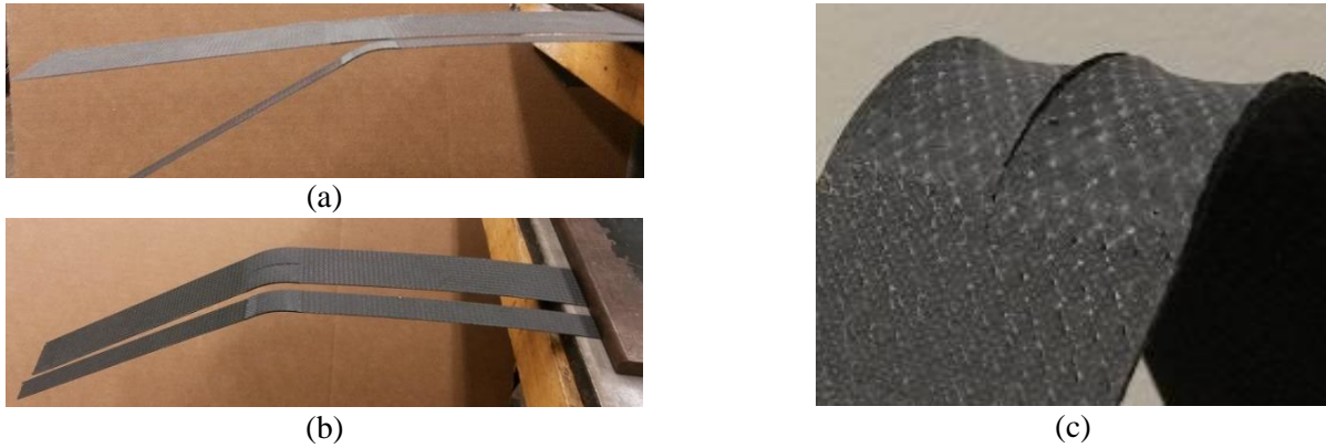
Figure 4. Bending stiffness comparison for (a) narrow and wide dual-matrix laminates, and (b) narrow laminate and wide laminate with a lengthwise slit in the elastomer region. (c) The anticlastic effect in a dual-matrix laminate.
