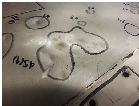
Figure 1. Dent cluster on a retired aircraft panel with dent impressions marked by inspection personnel
