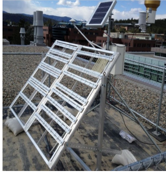
Figure 1: The set-up used for the natural ageing of test specimens
