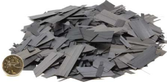
Figure 1. TET waste from Teijin Carbon America Inc. which has been chopped into strands following polymer impregnation.
