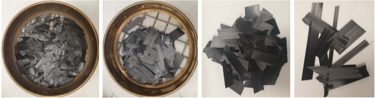
Figure 5. TET strand aggregates found in a number of different sieves following circular sieving trials.
