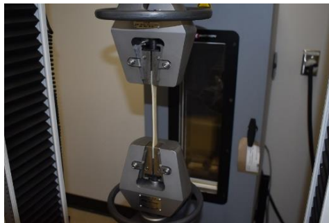
Figure 3. Coupon mounted inside the testing machine.
