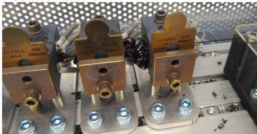
Figure 5: Polymer build-up at the entrance of the last die at the end of the study. Note the absence of such build-up on the second last die.
