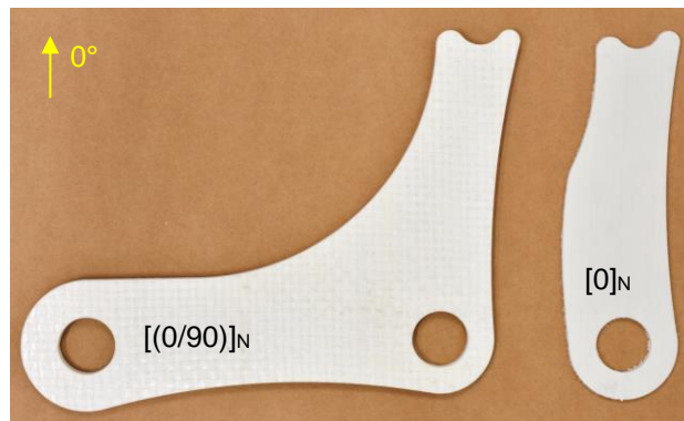
Figure 2. Thermoplastic composite inserts and lay-ups: full-skin (left) and localised skin (right) inserts
