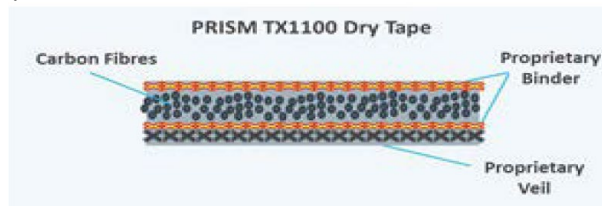
Figure 1. PRISM TX110 dry fiber tape cross-section [6]
