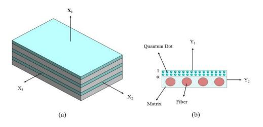
Figure 1: (a) Smart quantum dot-embedded laminated composite, and (b) corresponding unit cell.
