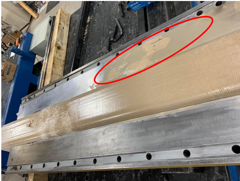
Figure 2. Resin Flow Out of The Die Cavity.
