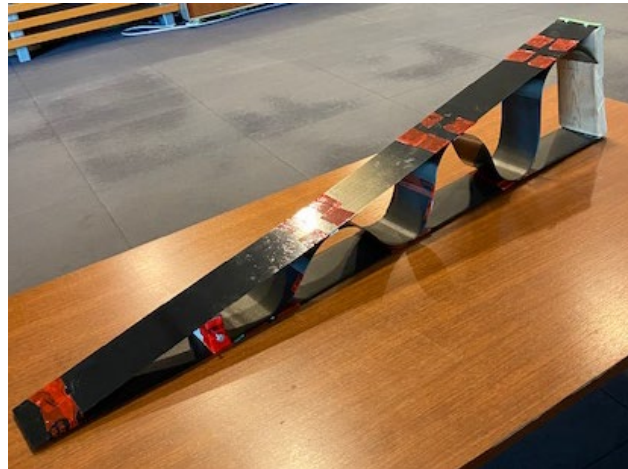
Figure 5: Sample of a flexible trailing edge made using 4D printing of composites
