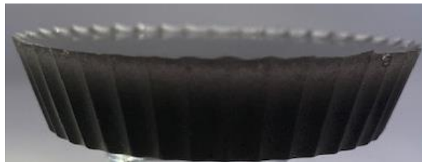
Figure 4. Filled polymer with a visible gradient (low concentration on top, high concentration on bottom)
