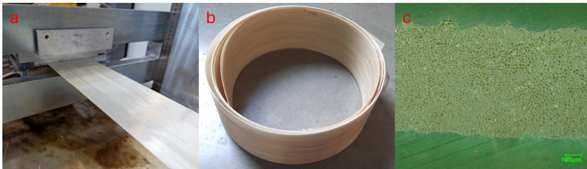
Figure 3. (a) Thermoplastic tape (67 vol% fiber content with 100 mm × 0.5 mm cross section) from melt pultrusion process exiting the die, (b) manufactured tape, and (c) microscopy of the tape cross section.
