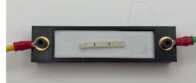
Figure 2. LCE actuator sample Joule heating test setup.
