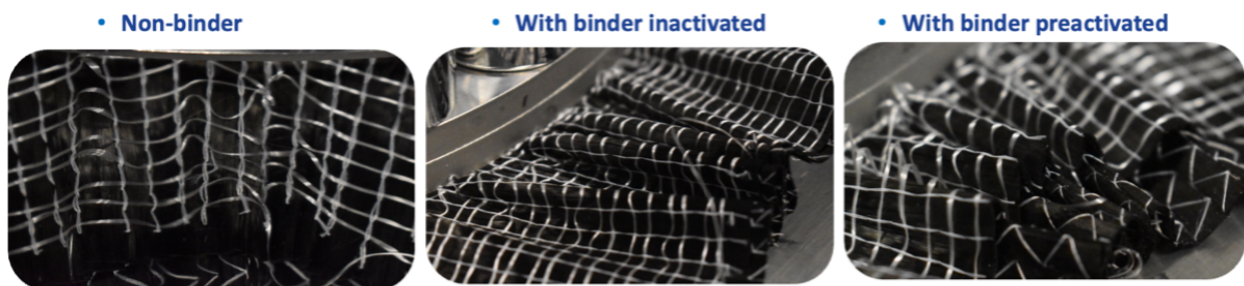
Figure 7. Representative fabric deformation at maximum punch displacement during double-layer hemispherical forming with stitch–stitch inter-ply interaction.
