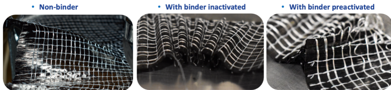
Figure 6. Representative fabric deformation at maximum punch displacement during single-layer hemispherical forming with the glass side in contact with the punch.
