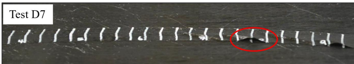
Figure 6. The folded wrinkle being measured in Figure 8. This test was conducted at a steering radius of 500 mm, a 40° C CFRP substrate, 50 mm/s deposition rate, and 100 N of compaction force applied with a compliant roller.
