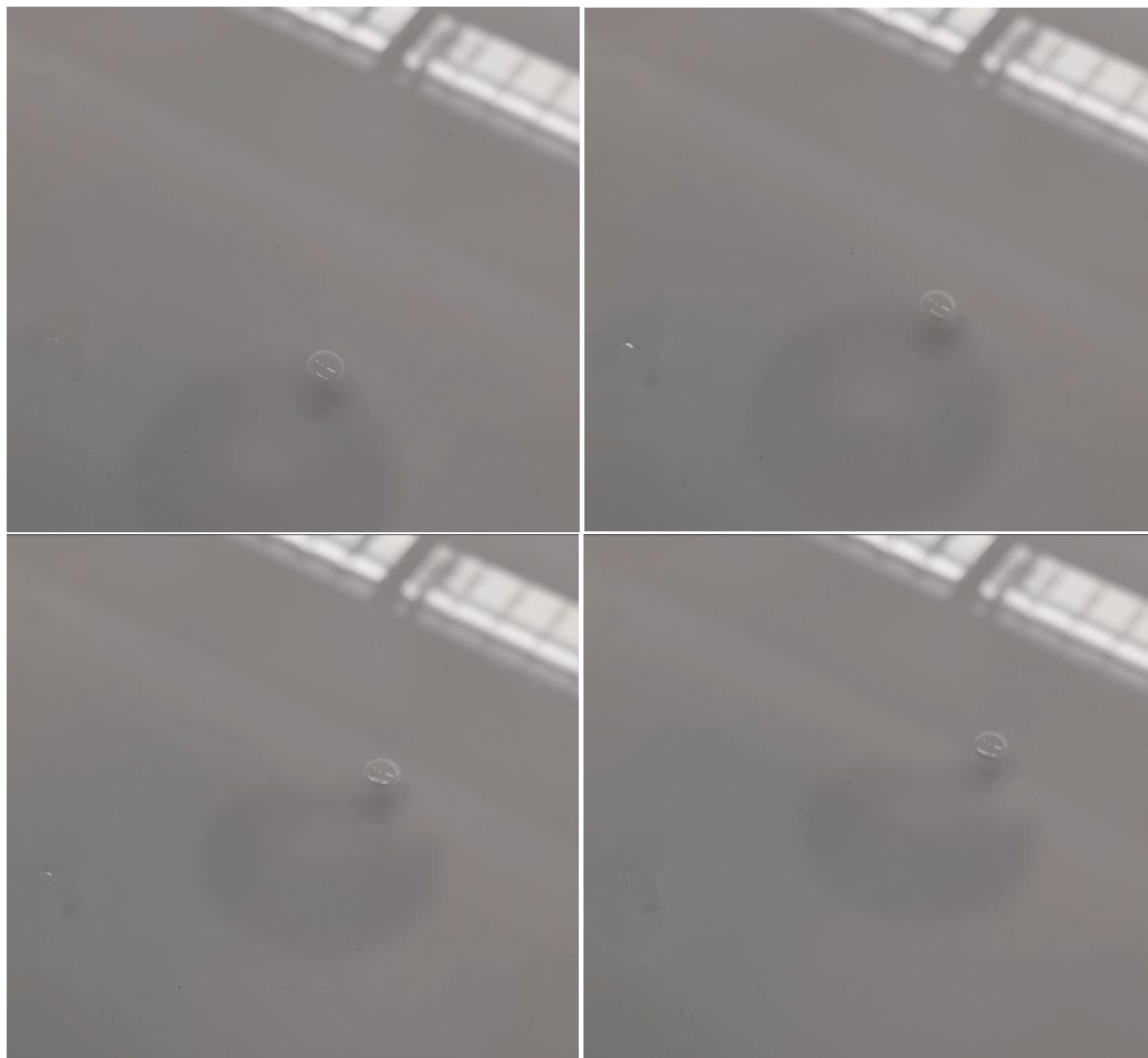
Figure 2: Temporal Evolution of Bubble Movement Due to Ultrasound. From Top Left to Bottom Right: t = 0, 2, 4, 6 s.
