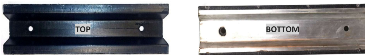
Figure 7. Experimental forming trials of an AISI 1080 steel-GF50/PA6 hybrid part.
