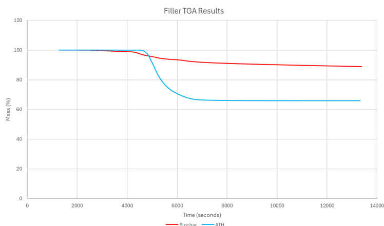
Figure 12. TGA results for fillers used in FR formulations.
