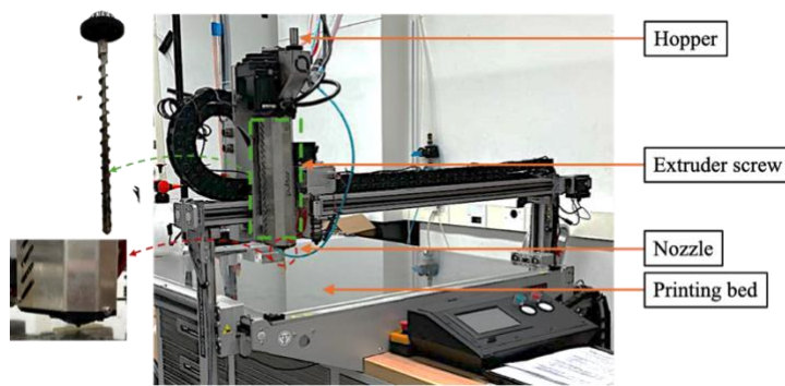
Figure 1 Schematic of the filament-free CBA-assisted 4D printing route
