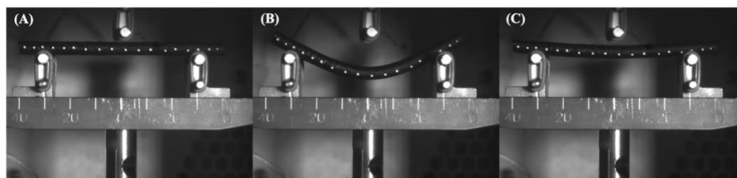
Figure 3 Representative shape-memory free-recovery of single-road deposited SMPU specimens: (A) original shape, (B) programmed temporary shape, and (C) recovered shape.
