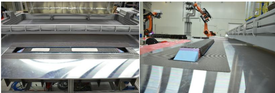
Figure 6. Detection of cut piece (top left), gripping of detected cut piece (top right), fiber angle measurement (center left), diaphragm draping (center right), foam core insertion (bottom left) and final preform (bottom right)
