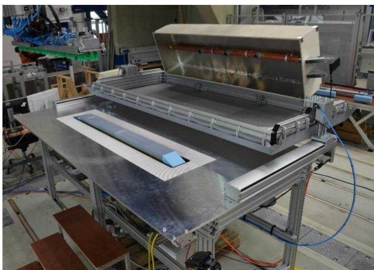
Figure 4. Preforming station for diaphragm preforming of patch preformed carbon fibers
