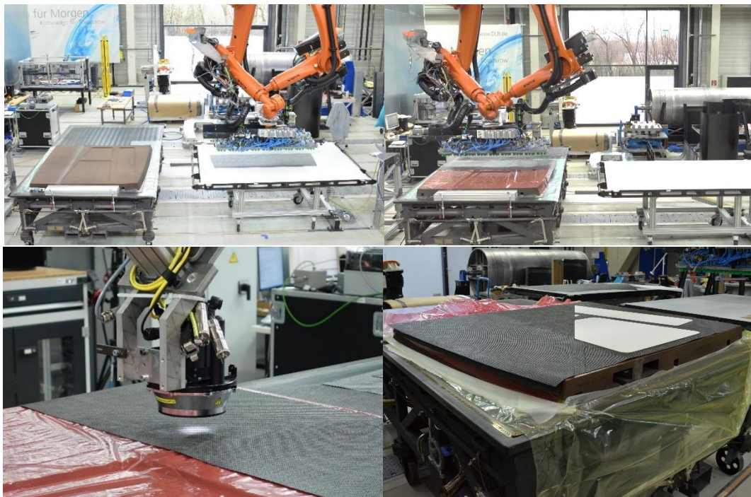
Figure 7. Cooperating gripping of cut piece (top left), cooperating transport and placement (top right), fiber angle measurement (bottom left) and foam core insertion (bottom right)
