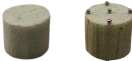
Figure 1: r-PET samples without perforation (left) and with 1.6mm diameter needles (right).
