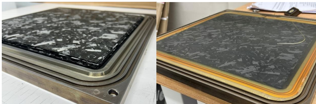
Figure 2: Discontinuous preforms stacked prior to infusion (left) with the resultant laminate after infusion (right)
