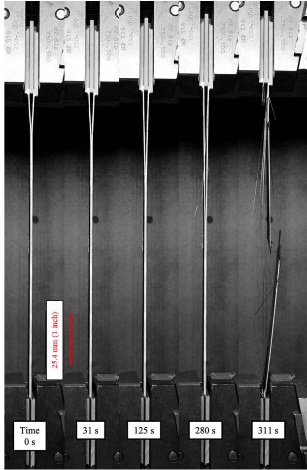
Figure 3: Crack propagation observed during the HOI test with an inserted tab thickness of 2.4mm.
