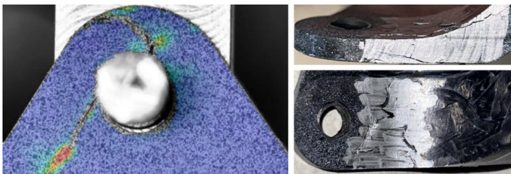
Figure 7. Typical Tension (Left) and Bending (Right) Fracture Surfaces
