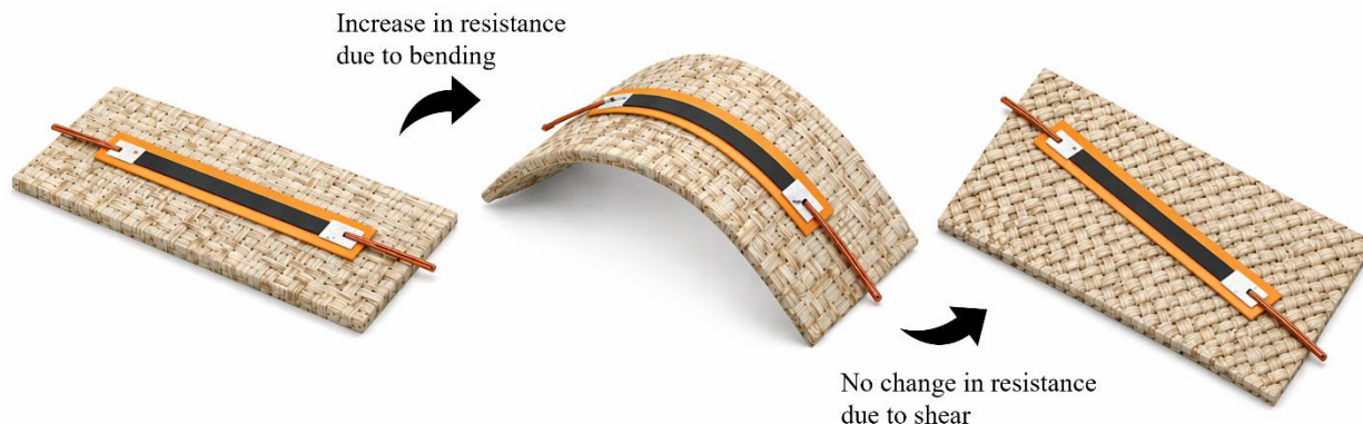
Figure 1 Schematic of the sensor working principle and how it changes resistance due to bending and shear deformation
