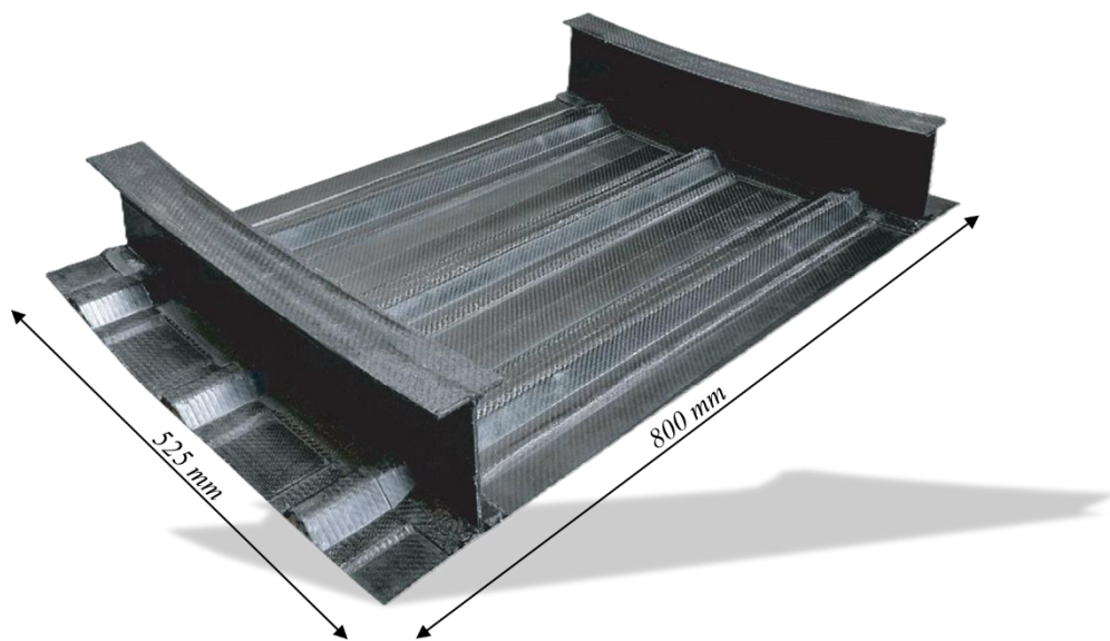
Figure 6. Curved CF RTP demonstrator panel with orthogonal stiffeners manufactured using one-step springback molding.
