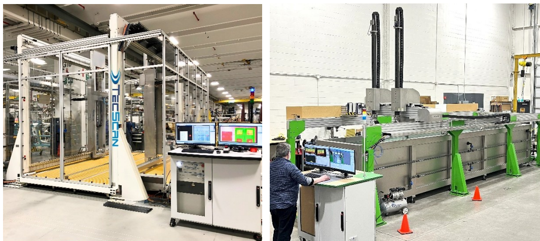
Figure 3. Gantry and Immersion platforms for inspection of complex composite aerospace structures.
