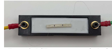
Figure 2. LCE actuator sample Joule heating test setup.
